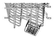
2. Rotate the upper sprayer and change the location of the container to ensure the upper sprayer is not obstructed by the 3in 1 tablet container. Refer to the figure below for reference.
